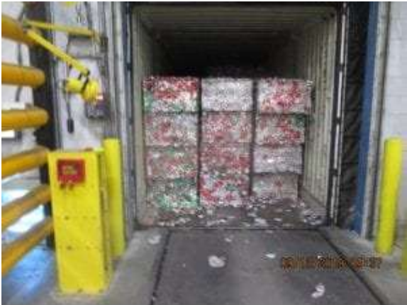
Small Compacted Bales Not Combined
