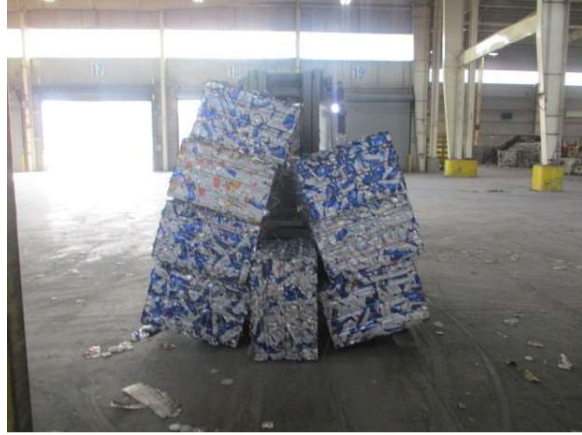
Multiple Small Bales Not Banded Together
