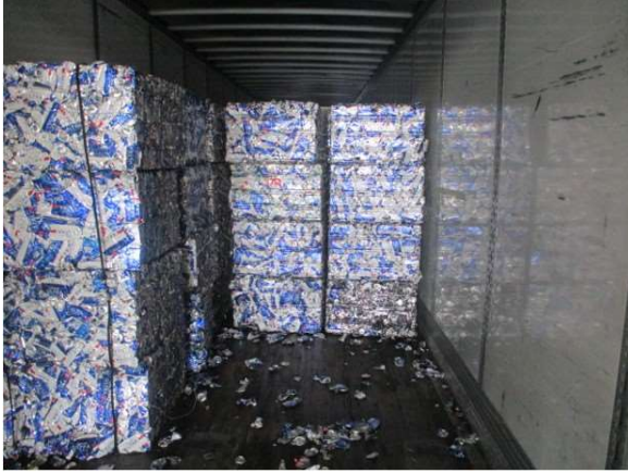
Multiple Small Bales Not Banded Together
