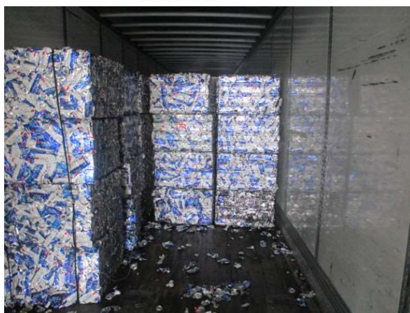
Multiple Small Bales Not Banded Together
