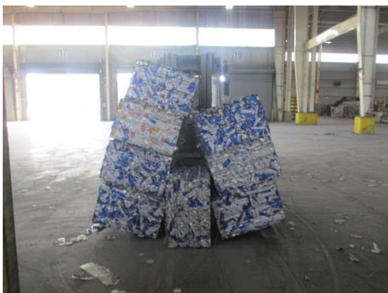
Multiple Small Bales Not Banded Together Class 3 Specification
