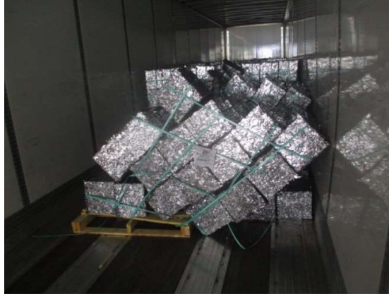
Improperly Secured to Pallet
