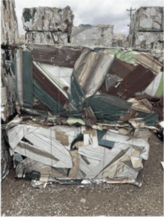
OPS – Baled with AT LEAST 4 wires
