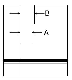
Gauge made from two pieces of steel with 2 bolts holding them together
