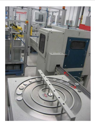
RSI samples are fed into the automated laboratory by the spiral magazine. Samples are automatically analyzed and then sorted.
