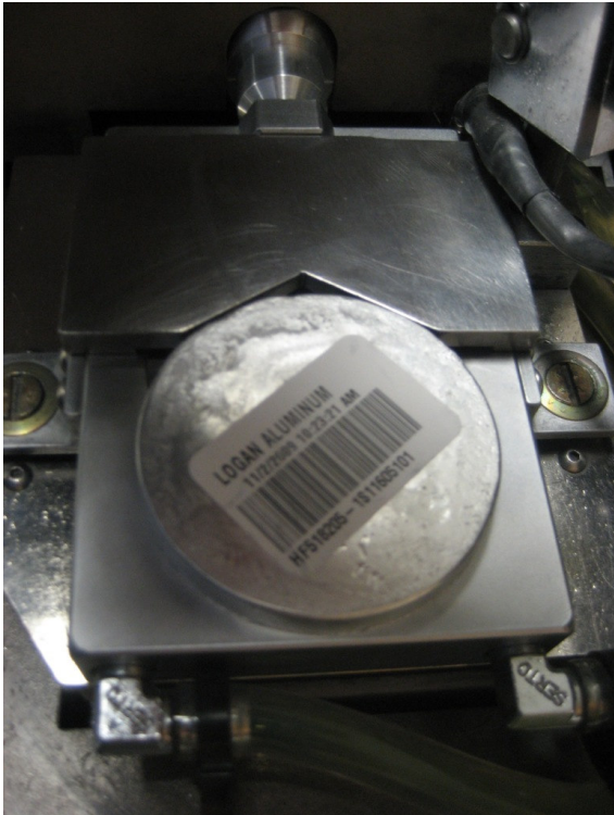
Example of spectrometer spark stand with sample backstop.
